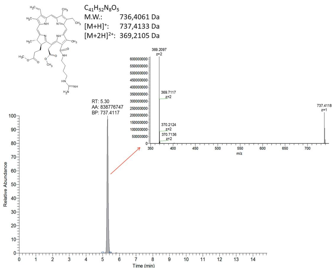
**Figure 3.** Mass chromatogram of a sample of guanidyl chlorin **2** from the reaction mixture. The retention time of the target compound is 5.30 min,  $m/z$   $[M+H]^+ = 737.4118$ ,  $[M+H]^{2+} = 369.2097$ .
