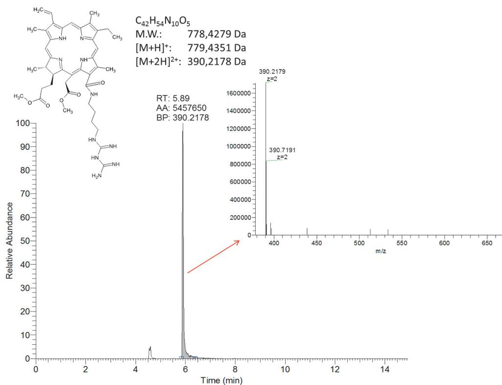
**Figure 4.** Mass chromatogram of a sample of the reaction mixture in the synthesis of  $13^2$ -(5-biguanidylbutylamido)-chlorin  $e_6$ . The retention time of the target compound is 5.89 min,  $m/z$   $[M+H]^{2+} = 390.2178$ .
