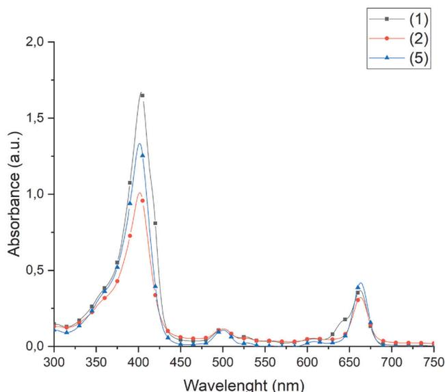
**Figure 1.** Absorption spectra of compounds **1**, **2** and **5**. The absorption spectra were obtained at the same solution concentrations and with dichloromethane as the solvent.
