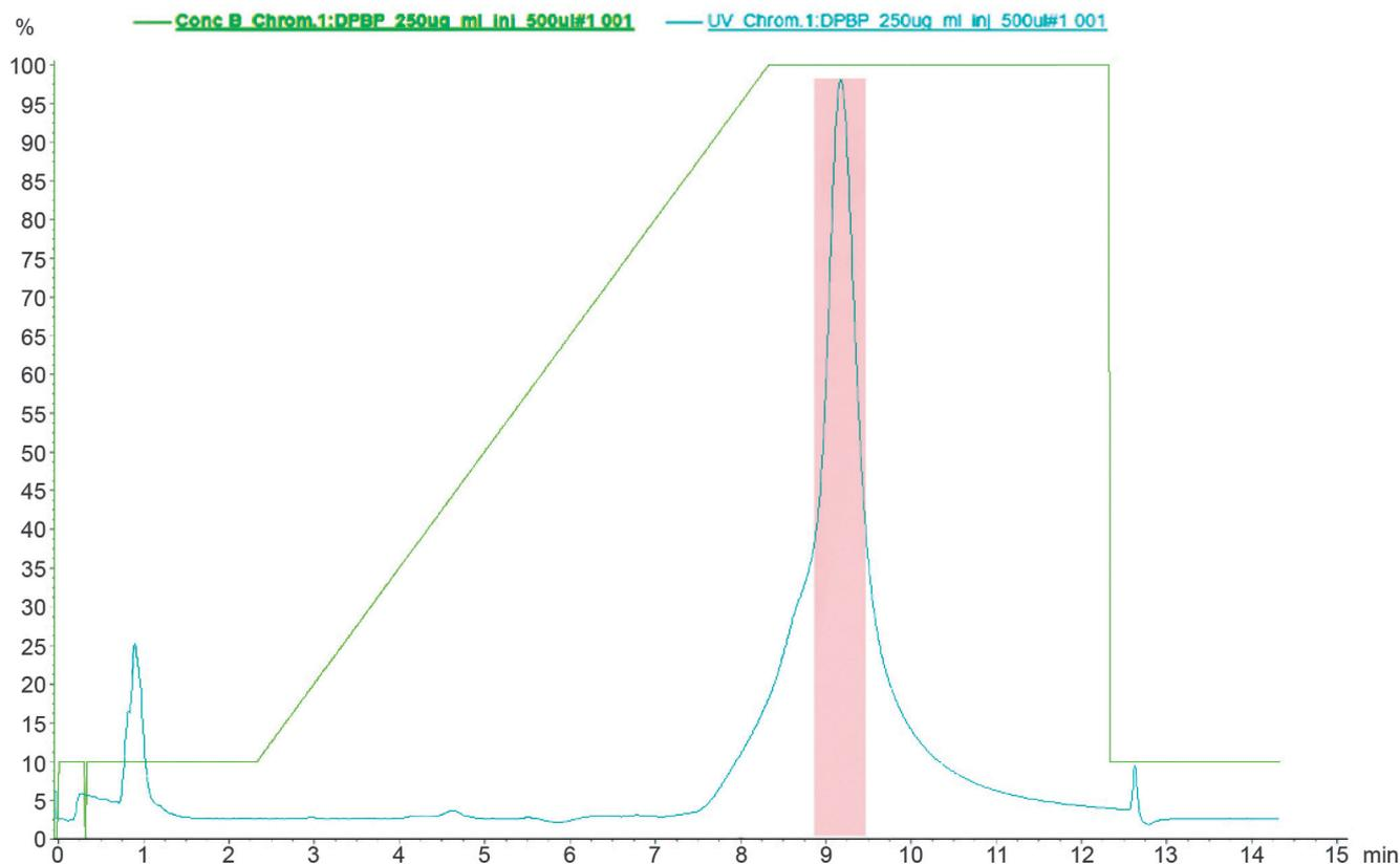
**Figure 2.** Chromatogram of preparative isolation of  $^{132}$ -(5-guanidylbutylamido)chlorin  $e_6$  from the reaction mixture performed using the “Acta Pure” chromatographic system.
