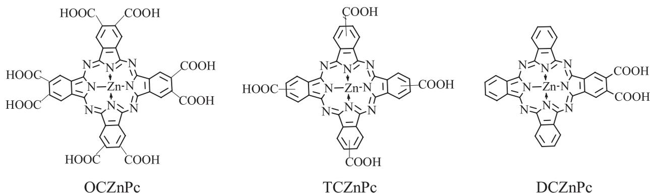
**Figure 1.** Structure of zinc carboxyphthalocyanines.
